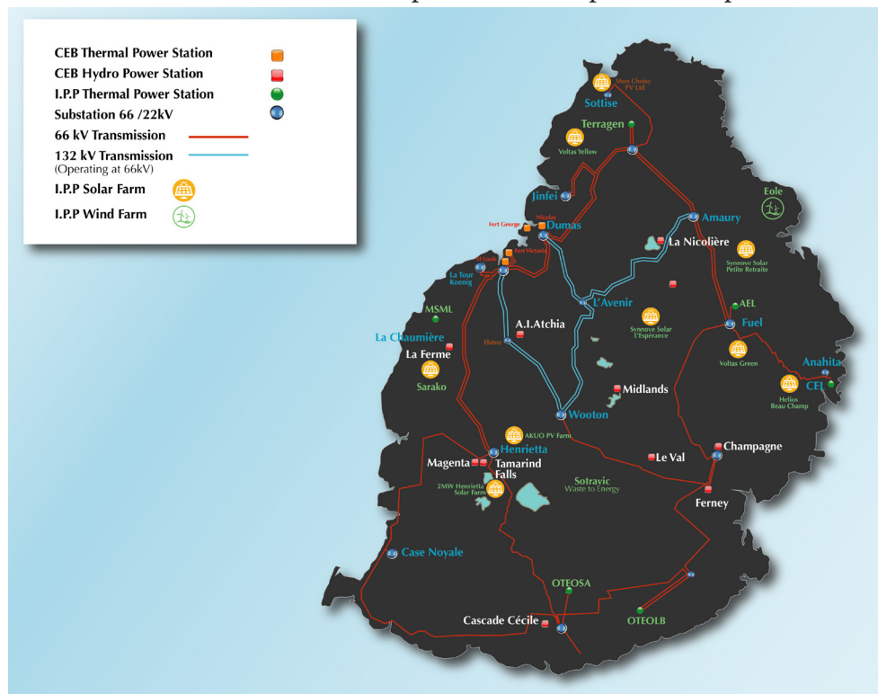
Figure 9: Central Electricity Board Network
